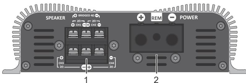
**1 - OUTPUT:** To connect the speakers. Follow the polarity and the minimum impedance recommended.
