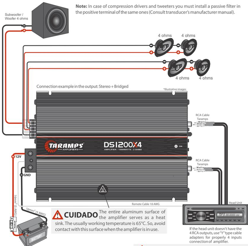
Examples of connections in the power supply input.
