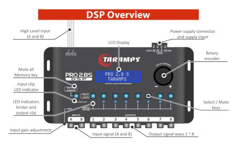
**Input gain adjustment:** With this adjustment in the MAXIMUM position, the DSP accepts signals of up to 2V RMS at the input. (Normal sensitivity). With the gain adjustment at MINIMUM, it is possible to apply signals from up to 9V RMS, without distorting the input. (Minimum sensitivity).
