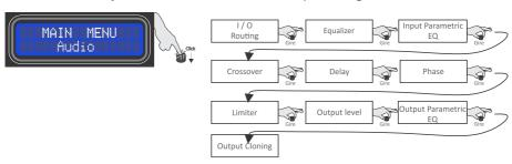
**I/O Routing:** Set the internal connections between outputs and inputs. Available options: A, B or A+B (sum of the two inputs).
