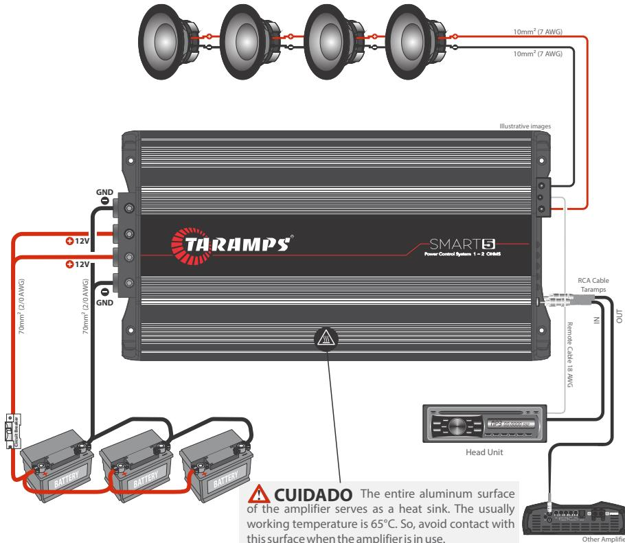
Examples of connections in the power supply input.
